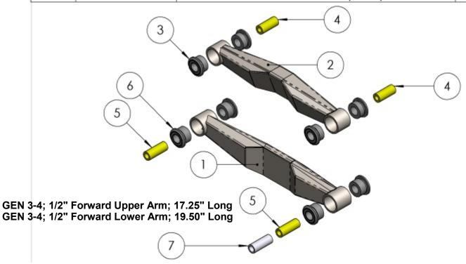
LUBE BUSHINGS WITH INCLUDED GREASE DURING ASSEMBLY. REUSE FACTORY BOLTS.
